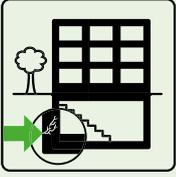
Cracks in the building substance are structurally weak points. Additionally, penetrating water may cause damage and may reduce the usage and lifetime of the building. An elastic sealing or structural-bonding of the crack is required. In order to achieve this, the crack is filled over its entire course with a polyurethane or epoxy injection resin via pressure injection.
